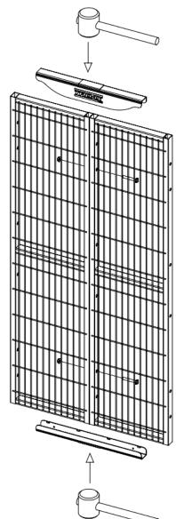
Snapper kit \$T30 29500221 Snapper kit \$T20 29500231 Includes one upper and one lower profile
